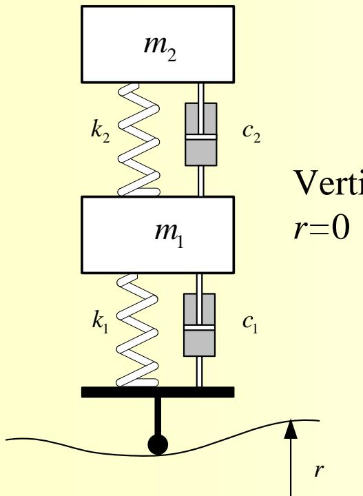
$$m_1 \ddot{y}_1 = -k_2(y_1 - y_2) - k_1(y_1 - r) - c_2(\dot{y}_1 - \dot{y}_2) - c_1(\dot{y}_1 - \dot{r})$$
