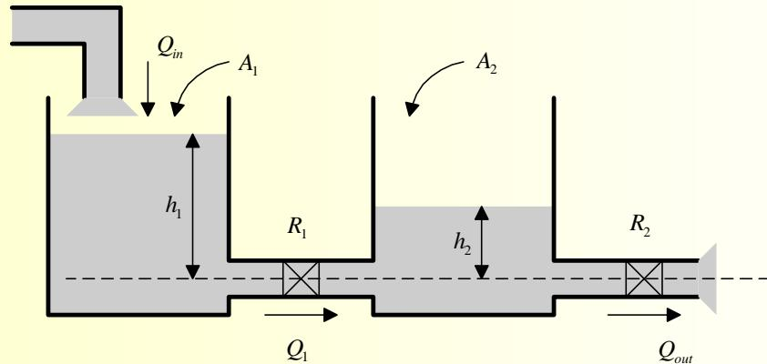
Derive the transfer function  $Q_{in} \rightarrow Q_{out}$  for the two tank system shown.
